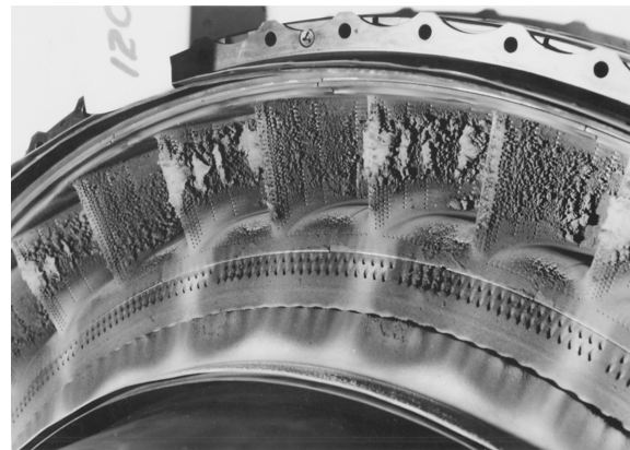
Fig. 3 Volcanic ash deposition on turbine vanes.
